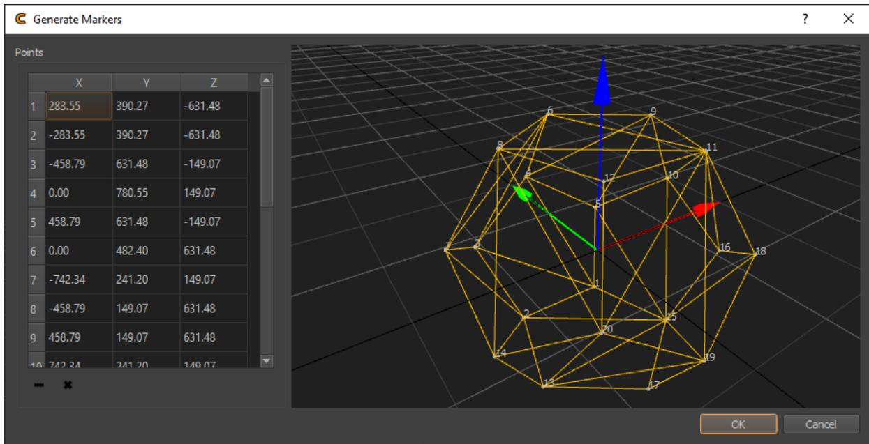
Measure points directly using a custom dialog and a Leica 3D Disto connected to the computer. See Pointer 3D *Pointer 3D* for further details.
