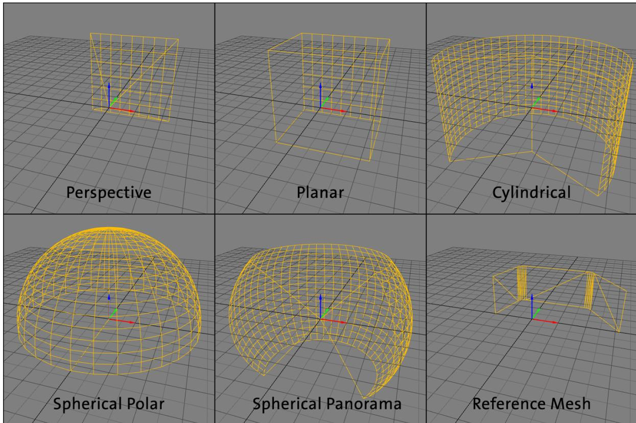
The mapping type reference mesh allows to import such 3d geometry from external files (e.g. obj, stl, ply, 3ds). The reference model should contain only one mesh with a continuous uv-mapping. It is recommended, that the reference mesh is larger than the used screen, to ensure that mapping is defined for the whole projection area.
