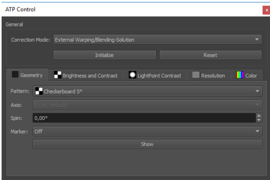
The ATP Control provides advanced test patterns usually required during Acceptance Test Procedure (ATP).
