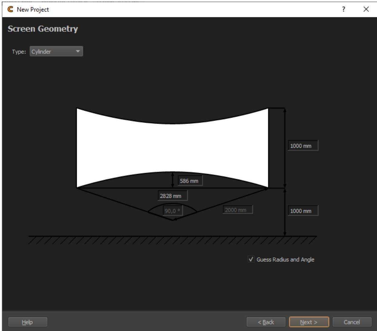
Fig. 2: Screen Geometry
