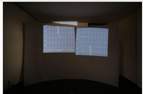
Warping assigned to corresponding outputs
