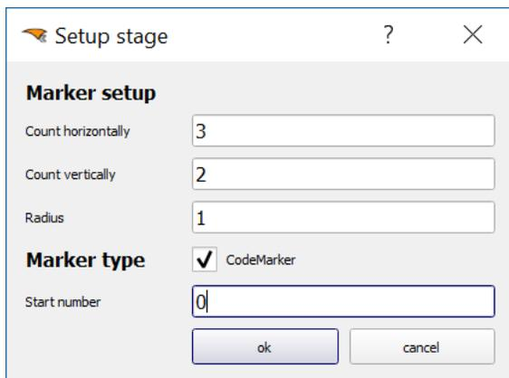
Markers can be moved by dragging in the central widget. A live preview is shown on connected PatternGenerators.
