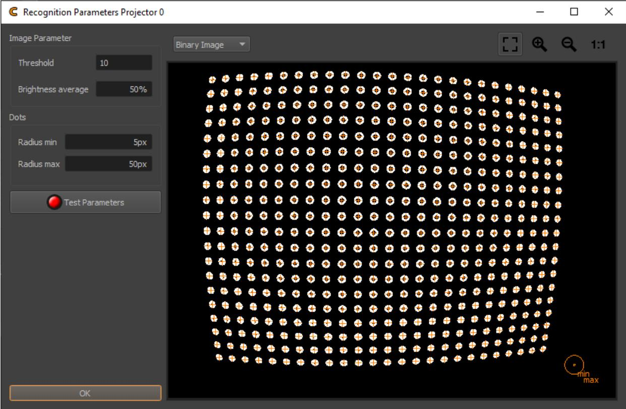
Fig. 10: Recognition Parameters Projector
