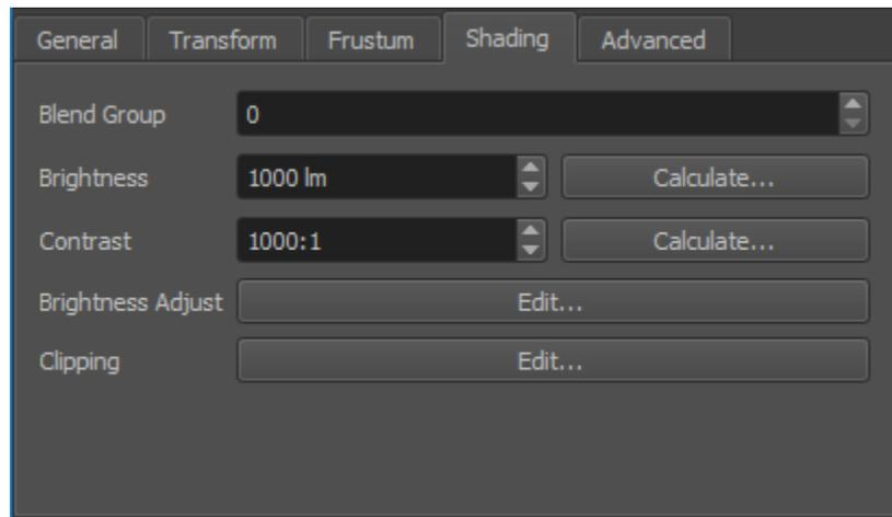
Fig. 6: Shading settings
