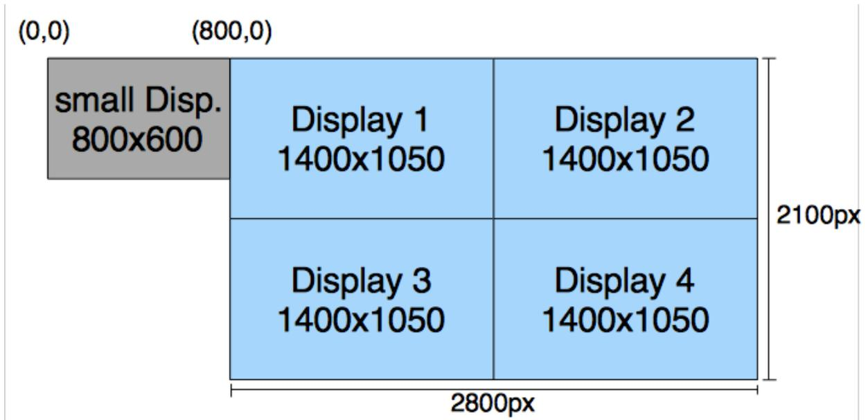
When all displays are visible to windows, the automatic mode **Secondary Displays** can be used.
