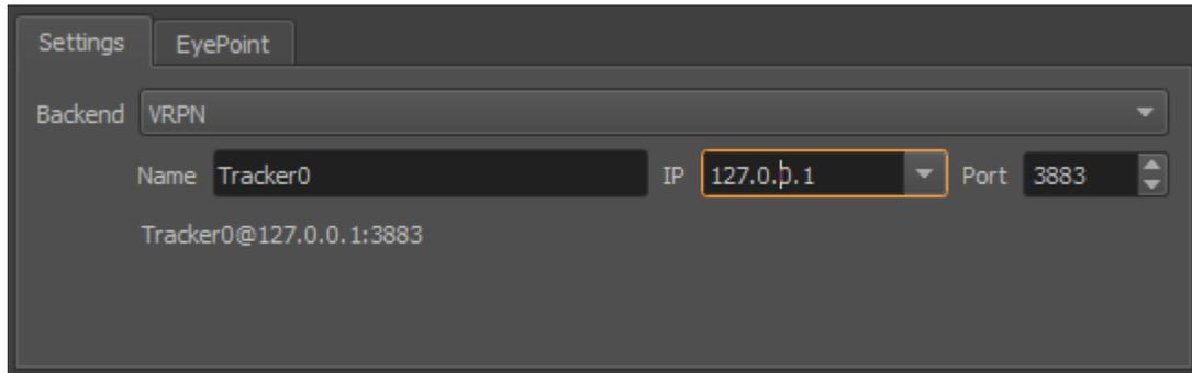
To enable the VRPN Tracker Simulator switch the Backend to VRPN. Then configure the VRPN tracker by selecting the name, IP address and port the Tracker Simulator should run on. Below the IP address drop down list you will find the identifier to be used in a VRPN client application.
