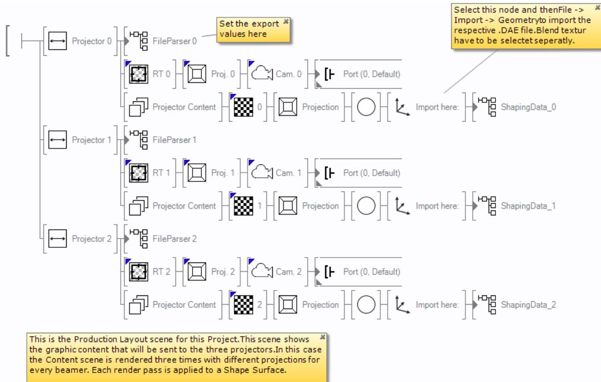
In order to import the warping correctly, following values have to be changed to set the proper field of view. The first thing to do is to import the `frustum_value.txt` file. To do so any of the fileParser nodes has to be selected to bring up the TxtFile node within the content window. There the text file can be chosen.
