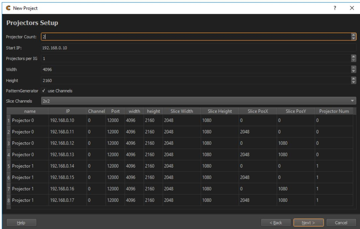
Activate “Slice Channels” with the required layout (1x2, 2x1 or 2x2). The channel list is generated accordingly. The generated list can be manually adjusted to change for example the ip-address of the individual sub-channels.
