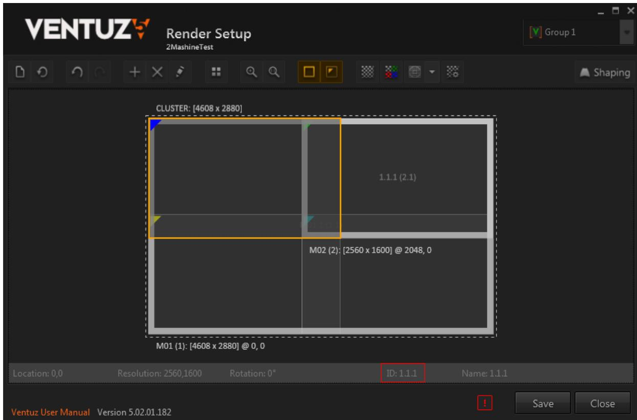
The cutting rectangles layout in Mapper2d must perfectly match the ventuz render setup, to get a matching result. Use to get unrotated cutting rectangles with defined overlaps.
