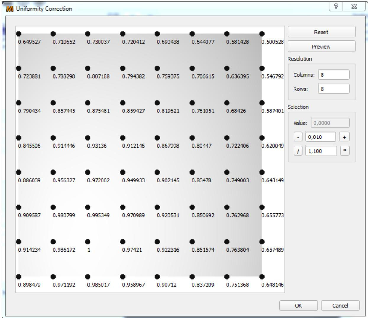
**Tip:** If a colorimeter is used for brightness measurements, the correction values can be directly derived from the luminance measurement differences.
