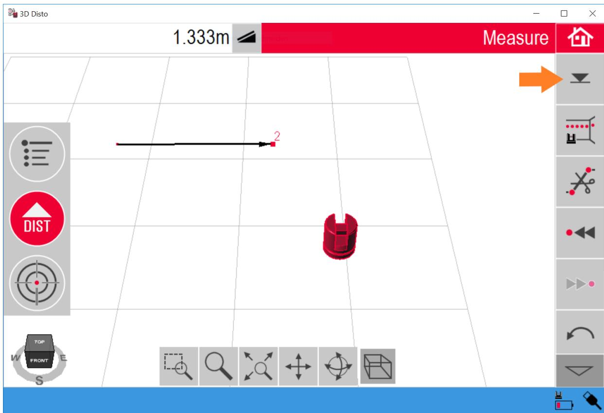
Fig. 1: Setting the reference height in the Disto 3D software
