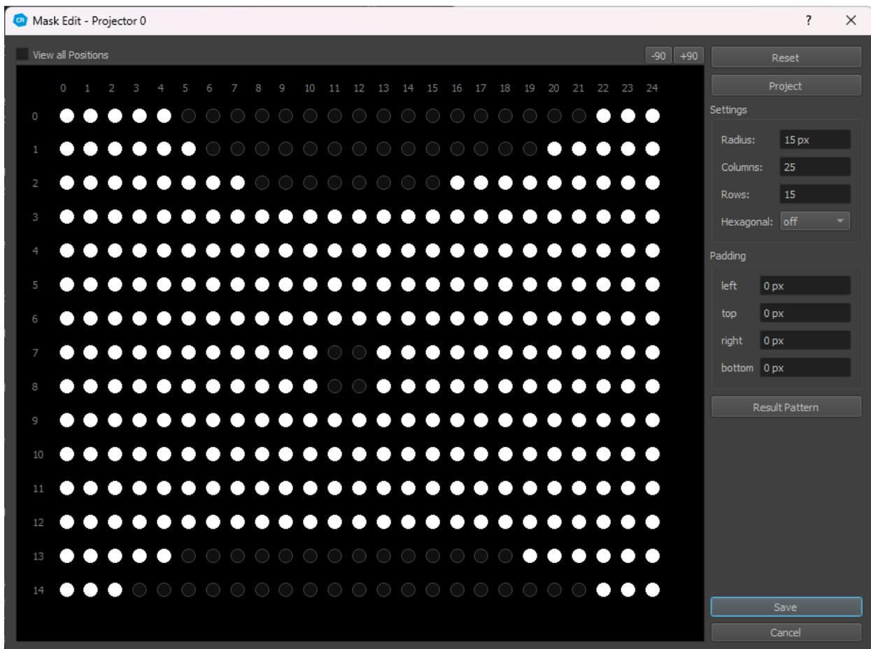
The Dot Pattern editor allows to reduce the projected points for a projector. This is often needed if points are projected beyond screen or only visible by half.
