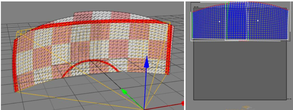
Straight image on screen and corresponding uv-coordinates after aspect correction.
