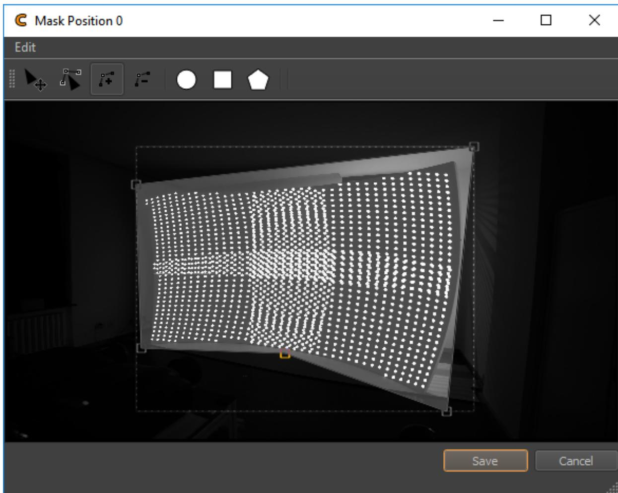
The masking is defined through the color of the background and the color of the shapes. Black areas are masked out. By default the background is white and created shapes are black, so that the created shapes cut out parts from the projection.
