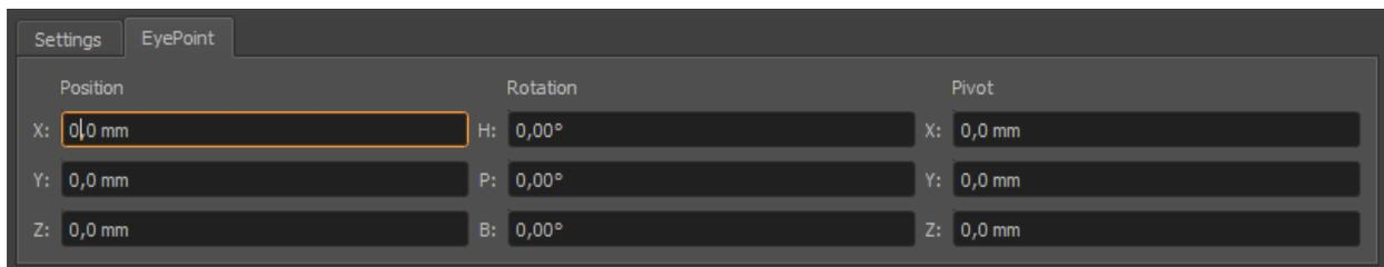
On the EyePoint page the eye point can be moved to any arbitrary point in 3d space as well. In addition the rotation and pivot can be defined as well.
