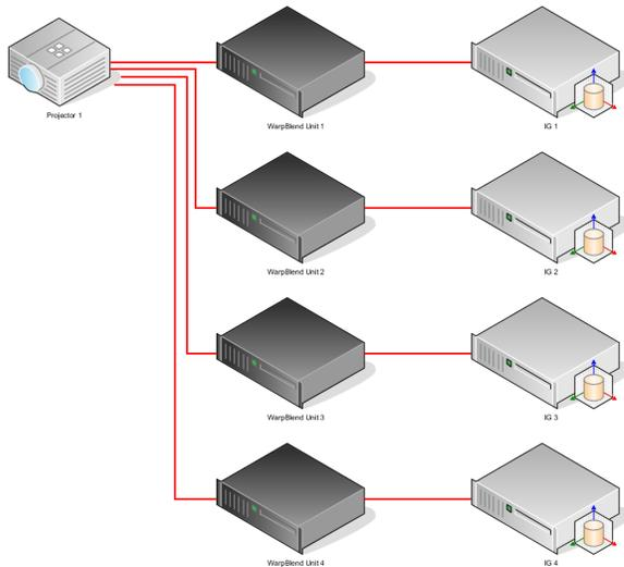
3. Projector is fed by multiple computers, with only **one warping/blending set for the whole projector** needed. Use **Sliced Channels** (see section *Sliced Channels*).
