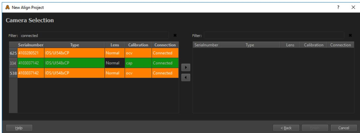
Select cameras in the left list that should be used in the align project. The list can be filtered for connected cameras, by entering "connected" in the filter.
