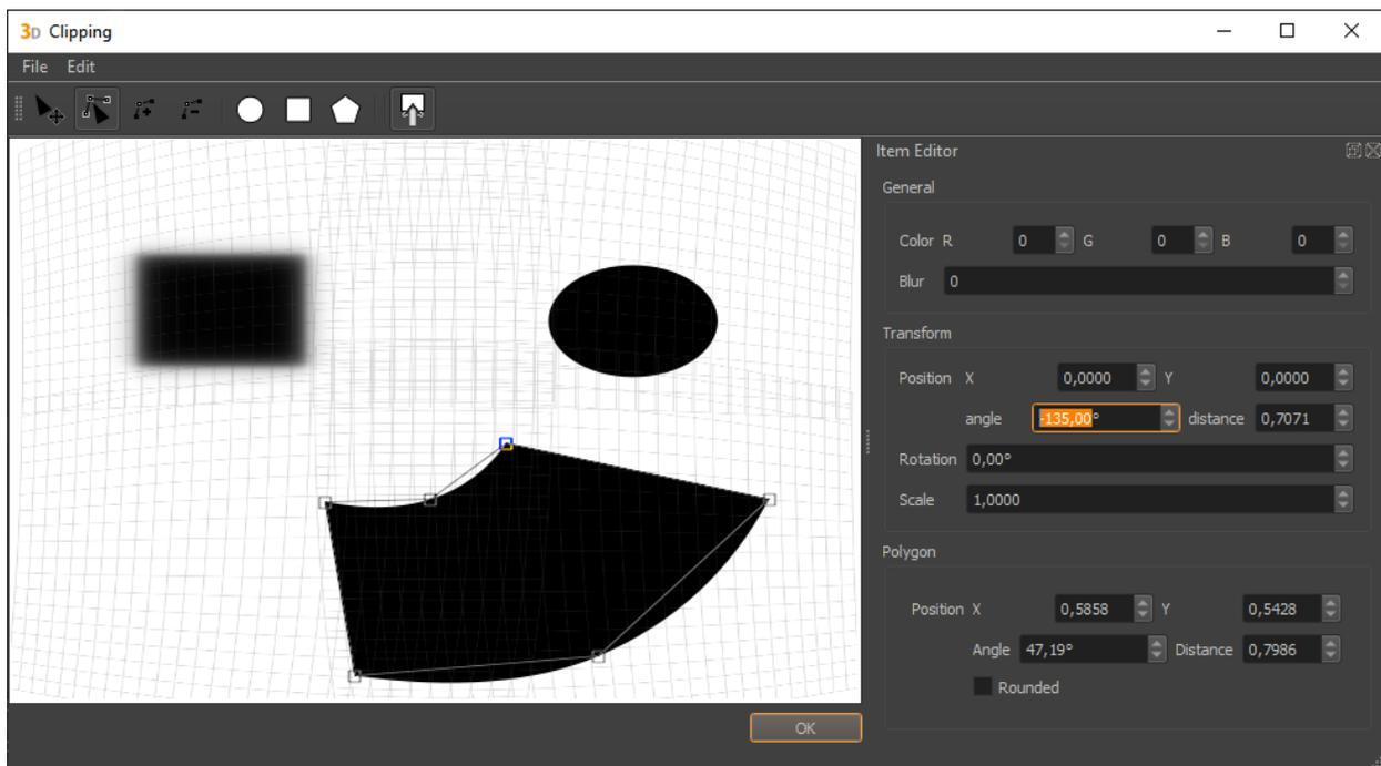
The Clipping Editor is used for vector based drawing of clipping images. The data is stored resolution independent and can be exported in varying resolutions. It supports a live-preview on the actual projection using the PatternGenerator.
