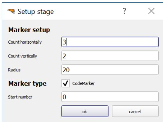
A new MarkerMover setup is created using this dialog.
