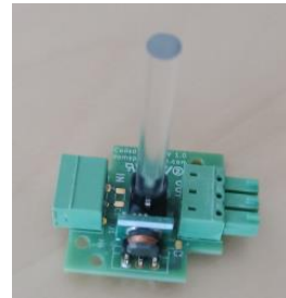
Figure 4 Coded LED Marker PCB
